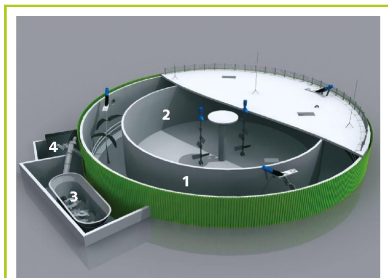
1 Main fermenter 2 Post fermenter 3 Feed system 4 Central pumping station
